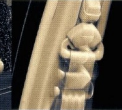
Front outboard shoulder belts have D-ring height adjusters to satisfy comfort for short and tall people alike.
