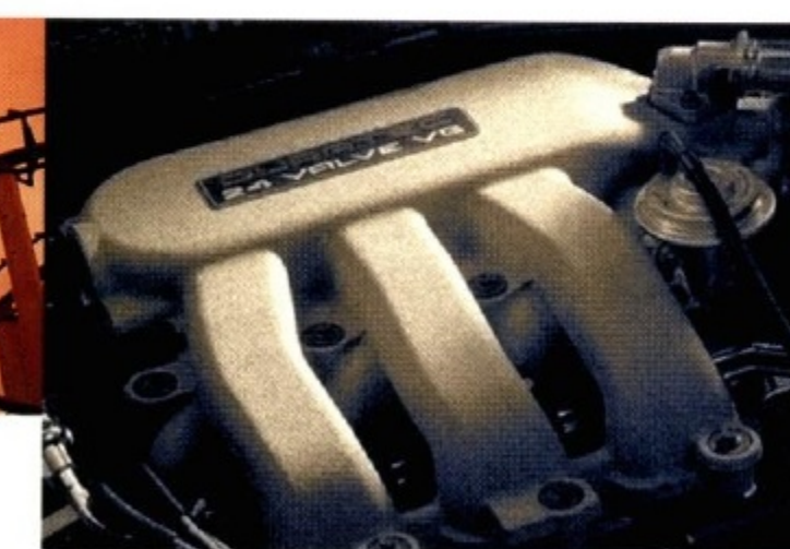
The potent 200-hp, 24-valve, DOHC 3.0-liter Duratec V6.
