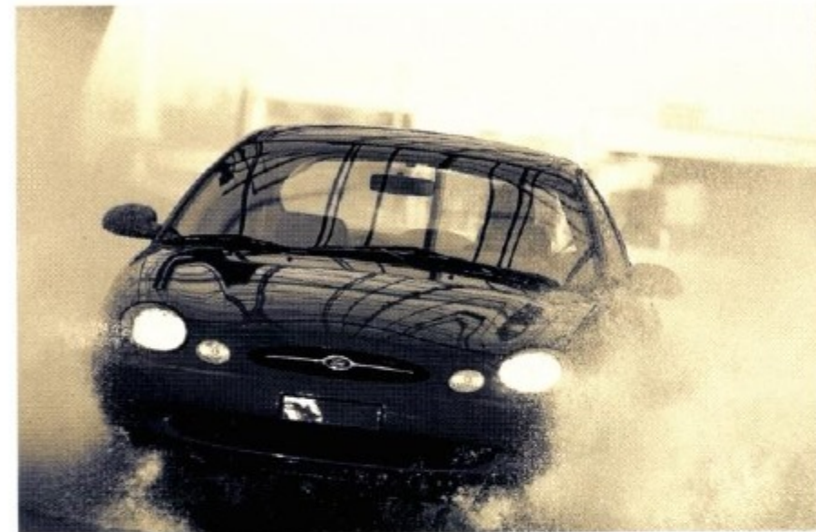
The 40 mph saltwater drive tests Taurus' ability to ward off corrosion.
