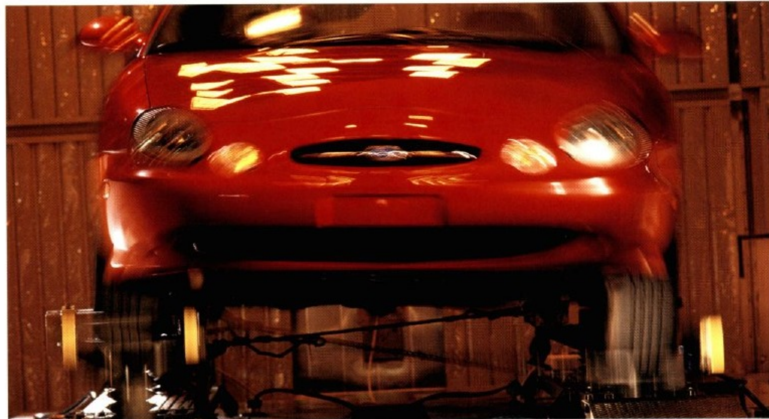
Testing prototypes for squeak and rattle, the 4-Post Shaker simulates 150,000 miles of wear and tear. With temperatures dipping as low as -40° F and rising as high as 180° F, the simulator is nearly as unforgiving as a family of four.
