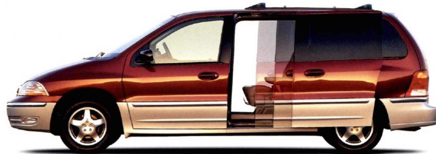
New available driver-side and passenger-side power sliding doors can be activated from two interior push-button locations and a remote key fob.
