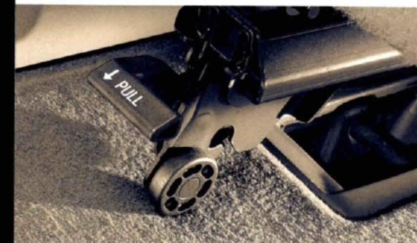
New available seat rollers on second-row and third-row bench seats make it easier to remove or install seats.*
