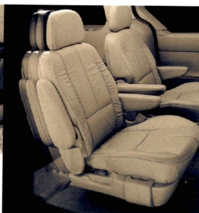
New second-row seat travel provides more leg room and easy entry for rear passengers.*
