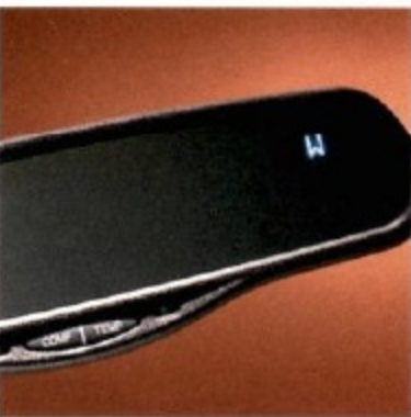
Electronic compass/mirror automatically dims when it detects glare from trailing headlamps.
