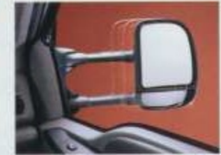
Available telescoping trailer tow mirrors (standard on chassis cabs) extend from the body for a better view. (Late availability.)
