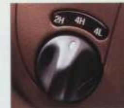
An electronic "shift-on-the-fly" system is available with 4x4s.
