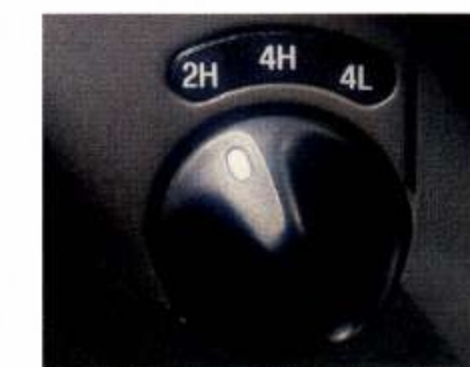
The electric shift-on-the-fly 4x4 system (optional with XLT and Lariat) has a rotary control switch for driver convenience.
