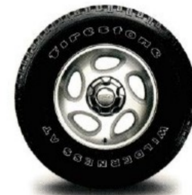
16" machined aluminum wheel, P255/70R16 OWL All-Terrain Tires (standard on Eddie Bauer, included in XLT Sport Group)
