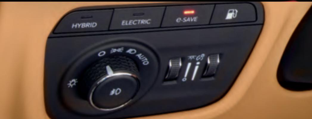
**YOU CHOOSE HOW AND WHEN TO OPTIMIZE THE AVAILABLE HYBRID DRIVETRAIN** via push-button controls on the dashboard. Select HYBRID for the best of both worlds, ELECTRIC to only use battery power, or e-SAVE to reserve battery power for later — like for low-emission zones in cities or driving through a majestic cedar forest — where you'll enjoy near-silent exploring with maximum torque and horsepower.
