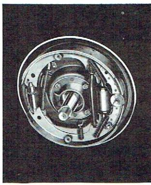
LaSalle's hydraulic brakes respond to light pressure. Moulded linings are moisture-proof.
