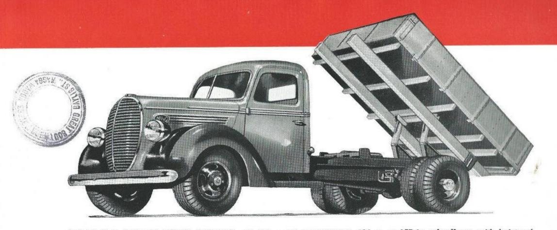
FORD V-8 HEAVY-DUTY TIPPER with G-Long Hydraulic Hoist, 134 in. or 157 in. wheelbase, with hoists of rated lifting capacity of 4 and 6 tons respectively. Hoist lifting arms are attached to body at four points, assuring safe lift on uneven ground. Extra rugged frame construction: 2-speed rear axle standard on  $4\frac{1}{2}$ -Ton models.
