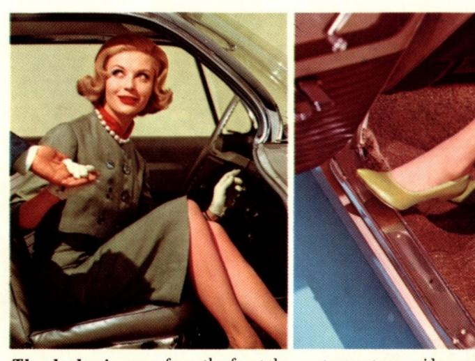
The dogleg is gone from the front door entrance to provide nearly five inches more of diagonal entry room. Door sills are narrower, too, for easier getting in and getting out. And Buick's new Hide-Away Drive Shaft reduces the tunnel height to give the middle passenger more leg room to stretch out and relax.
