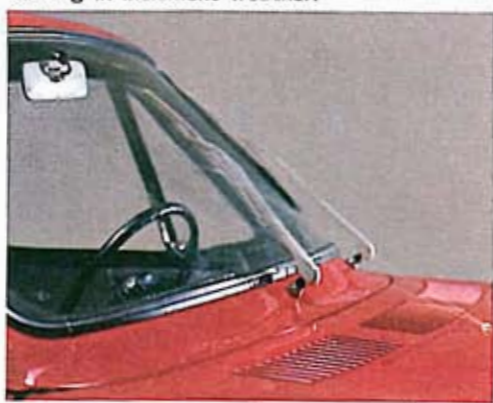
Windscreen Washer A stream of water lets the wipers clean mud or dirty spray from the windscreen quickly in rainy weather or on dusty roads.
