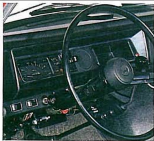
Soft Safety Padding Safety padding is incorporated in the steering wheel, dashboard, sun visor and rear of the front seat backs.
