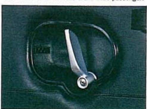
Recessed Door Handles Door handles are recessed and window control knobs are designed to prevent injury even if contacted smartly.
