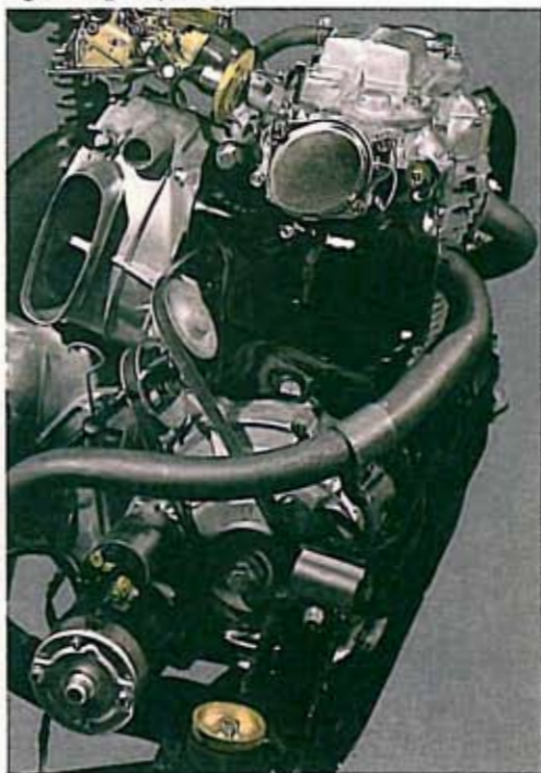
Low Load Fan Belt The fan belt is lightly loaded for long life, driving only the fan itself with all other accessories such as the generator being driven by gears.
