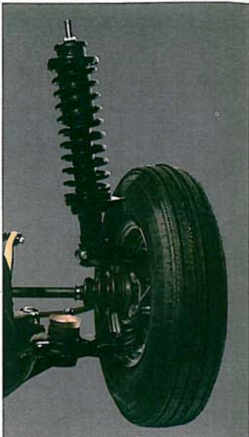
Front Suspension The superior strut type independent suspension utilizing struts, coil springs and shock absorbers is employed.
