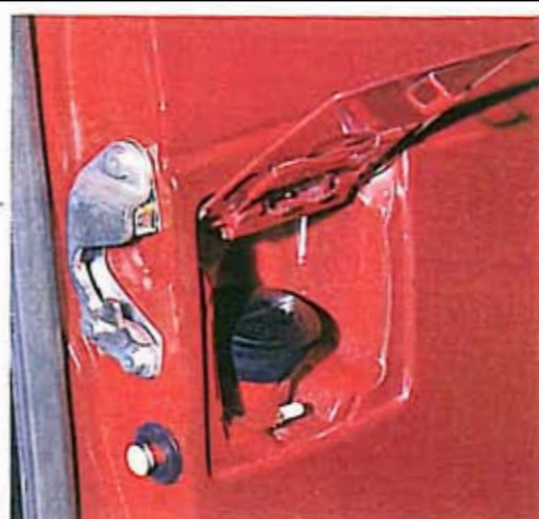
Shock-proof Latches Doors will not burst open and allow the occupants to be thrown out and injured in the event of an accident. The filler cap cannot be removed when the door is closed.
