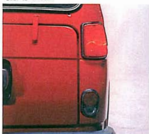
Reversing Lamps Large white rear lamps turn on when in reverse gear and throw a bright reversing light so objects behind car can be seen.
