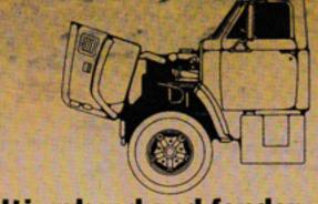
Tilting hood and fender assembly speeds engine maintenance procedures.
