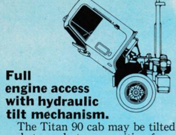
The Titan 90 cab may be tilted and stopped at any position from zero degrees to full tilt. Engine and front-end components are fully exposed for easy service. Hydraulic mechanism makes tilting a oneman job. All controls are mounted on the right-hand frame rail, away from traffic. Both mechanical and hydraulic latches protect against unwanted tilting.
