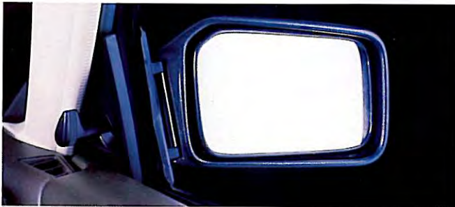
Large interior controlled mirrors
