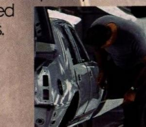
An inspector goes over a randomly selected vehicle inch-by-inch to check on fit and finish.
