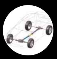
Locally built and calibrated for Australian conditions, this intelligent system enhances drive away acceleration, overall stability, grip and cornering control for safer, more spirited driving. And to complement the QuadTec<sup>™</sup> AWD system, the Verada AWD has improved high performance brakes, with bigger ventilated front and rear discs and front twin piston callipers.
