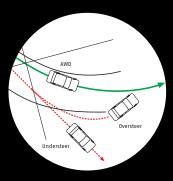
Using many elements from the famed rally-bred Mitsubishi Lancer Evolution, the QuadTec™ AWD system boasts superior roadholding and outstanding traction, which you can actually feel. Verada AWD has a refined AWD system which distributes torque evenly to all four wheels, however if it detects slip in any of the wheels the Viscous Coupling Unit regulates the torque to ensure that the car continues to corner efficiently, maintaining stability and power.
