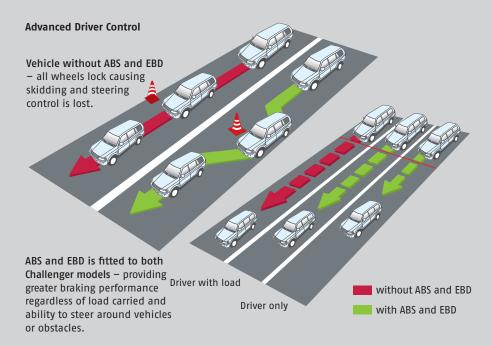
The 4 sensor, 4 channel Anti-lock Braking System (ABS) helps the driver maintain steering control, while Electronic Brake force Distribution (EBD) allows optimum straight line stopping control and minimum stopping distance regardless of the number of passengers or payload.
