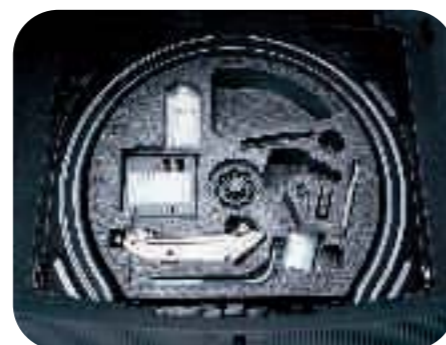
● tire mobility system with 12 volt compressor and tyre sealant, stowed under the load floor cover in the luggage compartment; optional space-saving spare wheel
