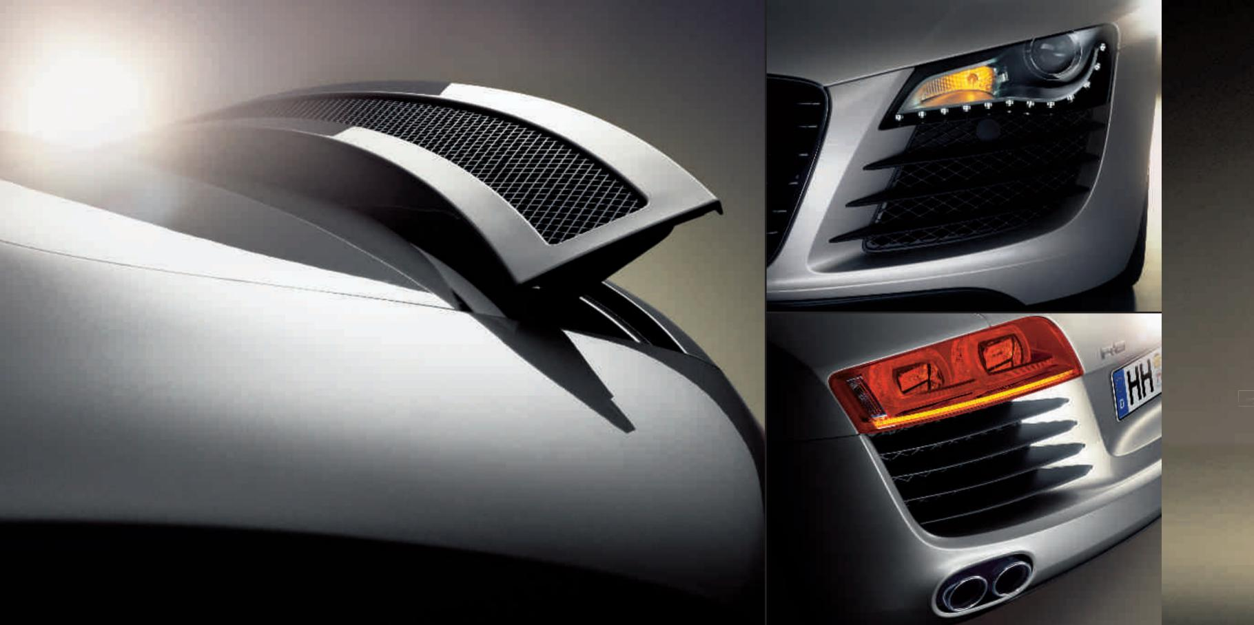
The rear spoiler is automatically extended at 100 km/h and is retracted sleekly back into the vehicle silhouette at 35 km/h. The spoiler can also be activated by pressing a button.
