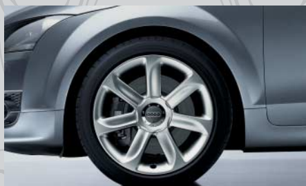
Cast aluminium wheels in 7-arm styling, 9 J x 18. >8J-7-006 500* 8J0 601 025Q 8 J x 18. 8J-7-006 501* >8J0 601 025AC centre cap (8J0601165A)
