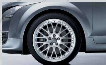
Cast aluminium wheels in 20-spoke styling, 9 J x 19. 8J0 601 025P centre cap (4B0601170A72J)
