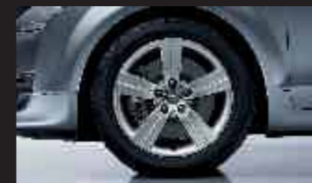
Cast aluminium wheels in 5-arm trapezoidal styling, size 8 J x 17 with 225/50 R 17 tyres (only for 2.0 TFSI)
