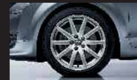
Cast aluminium winter wheels in 10-spoke styling, size 9 J x 18 with 245/40 R 18 V tyres, permissible top speed 240 km/h
