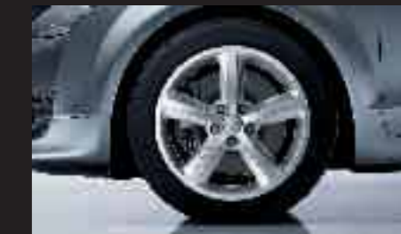
Cast aluminium wheels in 5-spoke styling, size 9 J x 18 with 245/40 R 18 tyres
