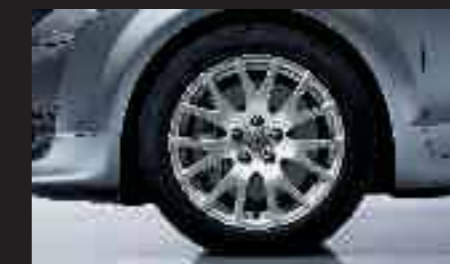
Lightweight forged aluminium winter wheels in 7-Y-spoke styling, size 7 J x 17 with 225/50 R 17 H tyres, permissible top speed 210 km/h
