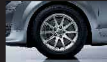
Cast aluminium wheels in 10-spoke star styling, size 7.5 J x 16 with 225/55 R 16 tyres (standard for 2.0 TFSI)
