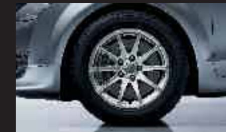
Cast aluminium winter wheels in 10-spoke star styling, size 7 J x 16, with 225/55 R 17 tyres 16 H, permissible top speed 210 km/h (only for 2.0 TFSI)
