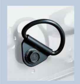
A cargo protection bar and cargo tie down rings, prevent loose loads from moving around in transit.
