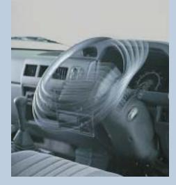
Tilt adjustable steering wheel provides comfort to help prevent driver fatigue.
