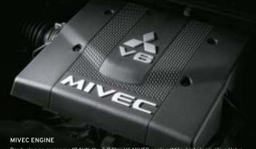
Producing an awesome 184kW, the 3.8 litre V6 MIVEC engine (Mitsubishi Innovative Valve timing and lift Electronic Control) delivers unbelievable power for a sports 4WD. MIVEC offers the latest intelligent valve-timing technology to deliver improved fuel efficiency and lower emissions, while providing improved driveability. The MIVEC engine matches your driving style to minimise fuel consumption at lower revs while increasing airflow at high revs for greater performance.
