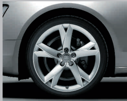
Cast aluminium wheels, 5-arm Y design, size 8.5 J x 19 with 255/35 R 19 tyres
