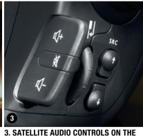
3. SATELLITE AUDIO CONTROLS ON THE STEERING WHEEL enable you to select tracks and radio frequencies, adjust the volume, store settings and play CDs.
