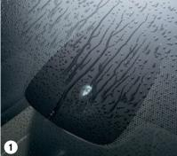
1. LIGHT AND RAIN SENSORS located on the windscreen activate the headlamps automatically if light levels drop, or start the front windscreen wipers in the event of rain.
