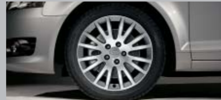
Cast aluminium wheels, 16-spoke design, polished, two-colour, size 7.5 J x 17 with 225/45 R 17 tyres
