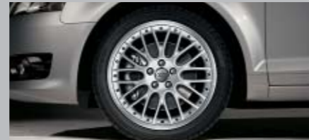
Audi exclusive cast aluminium wheels, 20-spoke design, two-piece, size 7.5 J x 18 with 225/40 R 18 tyres. From quattro GmbH
