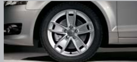
Cast aluminium wheels, 5-arm design, size 7.5 J x 17 with 225/45 R 17 tyres (exclusive for Ambition)
