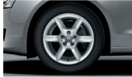
Cast aluminium wheels, 6-spoke parabola design 1 , size 8 J x 17 with 245/45 R 17 tyres
