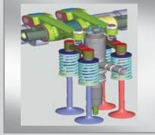
4 Valve Overhead Camshaft
