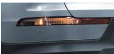
Turn-signal lamps are separately located from the lower rear lamp cluster to enhance visibility
