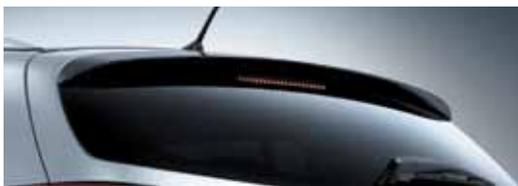
Rear spoiler & LED high-mounted stop lamp enhances the aerodynamics and brake light visibility
