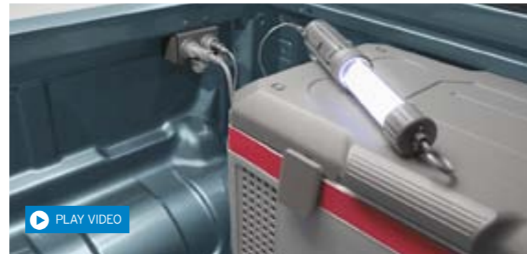
12 volt auxiliary sockets Contains two 15 amp sockets to provide power to small electrical items. (Utilities only.)
