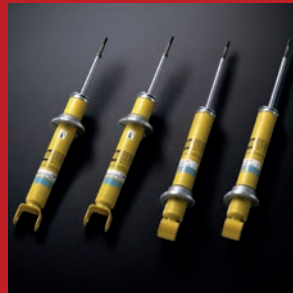
Bilstein shock absorbers (manual only).
