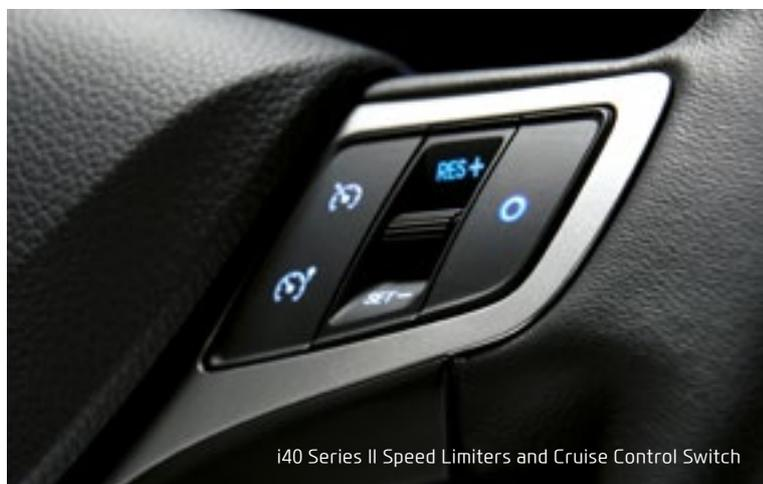
i40 Series II Speed Limiters and Cruise Control Switch
