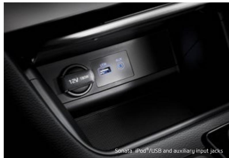
Sonata iPod®/USB and auxiliary input jacks
