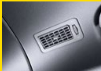
Air conditioning - dual zone system with roof mounted side vents for centre & rear
