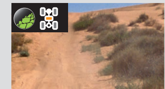
4LLC (4WD Low Range with locked centre differential) For steep hills, sand, deep snow, etc. ^
