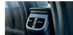
Rear cooling/heating vents
