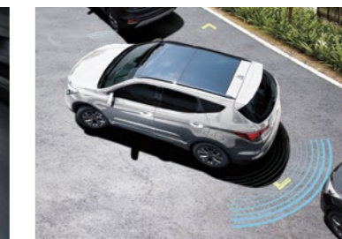
Advanced Smart Parking Assist System (ASPAS) The ASPAS which is only available on the Highlander variant, safely steers the car in and out of parking spots, in 'Reverse Parking(90°)', 'Parallel Parking' and Parallel Parking 'Exit' modes. All you need to do is operate the accelerator, brake and gear levers as necessary.
