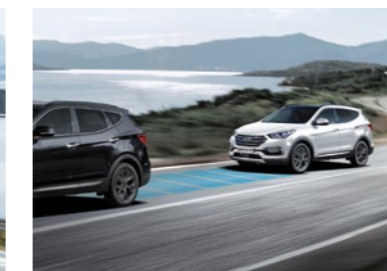
Smart Cruise Control (SCC) Automatically maintains distance from the car ahead, up to a preset speed. Car comes to a complete stop and restarts in 3 seconds once the car in front departs.
