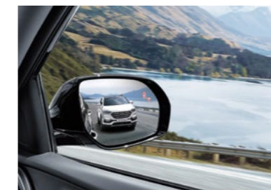
Blind Spot Detection (BSD) When driving at a speed of 30km/h or higher, the BSD function will alert the driver to vehicles that enter the blind spot, including during lane changes.
