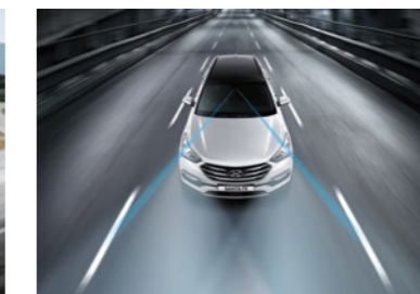
Lane Departure Warning System (LDWS) A camera mounted on top of the windshield of Highlander variants, provides a cutting edge preventive safety mechanism by recognising lane departures that are not accompanied by a turn signal, and then initiating an alert to the driver.
