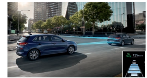
Smart Cruise Control (SCC) Automatically maintains speed and distance from the car ahead. Car comes to a complete stop and restarts in 3 seconds once the car in front departs.
