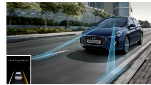
Lane Keeping Assist System (LKAS) Uses the front camera to detect lanes and helps prevent the vehicle from steering off the lane.
