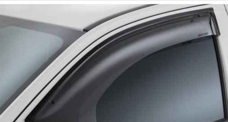
WEATHERSHIELDS Made from UV-resistant acrylic, weathershields let fresh air in while keeping the elements out. (Front only)
