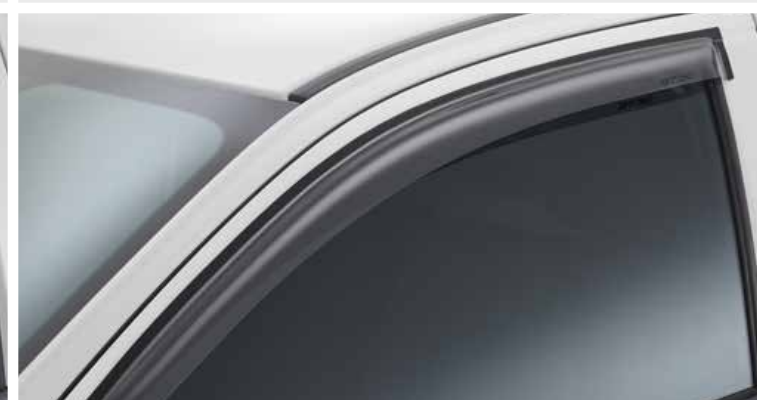
SLIMLINE WEATHERSHIELDS Allow fresh air into the cabin whatever the weather, allowing heat to escape and preventing windows from fogging. (Set of two or four)
