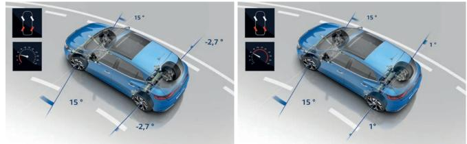
At speeds below 60km/h (below 80km/h in Sport mode), the rear wheels At higher speeds, the rear wheels turn in the same direction as the turn  $2.7^{\circ}$  in the opposite direction of the front wheels.
