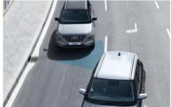
Blind-Spot Collision Warning (BCW)<sup>2</sup> When driving at a speed of 30km/h or higher, the BCW function will alert the driver to vehicles that enter or are in the blind spot, to help avoid potential collisions during lane changes.
