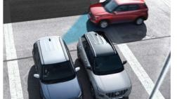
Rear Cross-Traffic Collision Warning<sup>2</sup> RCCW monitors for traffic approaching on either side of the Venue when reversing out of perpendicular parking spaces. Should RCCW detect a vehicle approaching, an audible warning will sound, with a visual warning displayed on the dash cluster.
