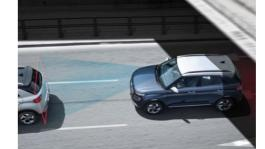
Forward Collision-Avoidance Assist (FCA) -City/Urban/Interurban/Pesestrian (camera type) Using camera data, the FCA system autonomously activates the brakes when it detects dangerous and sudden braking by the car ahead, or movement of pedestrians on the road.
