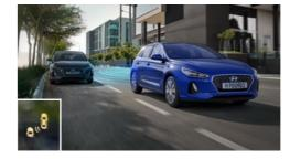
Blind-Spot Collision Warning (BCW) When driving at a speed of 30km/h or higher, the BCW function will alert the driver to other vehicles in the i30's blind spot, including during lane changes.
