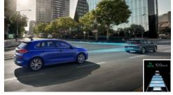
Smart Cruise Control (SCC) with Stop & Go Detects the speed and distance of vehicles ahead of the i30, and automatically maintains a safe distance to the vehicle ahead, up to a pre-set speed.
