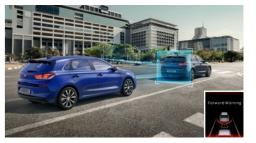
Forward Collision-Avoidance Assist (FCA) Combining radar and camera data, the FCA system autonomously activates the brakes when it detects potential collisions with vehicles, cyclists, or pedestrians in front of the i30.
