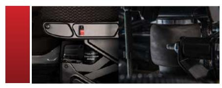
Layers of air between you and the bumpy road. Air suspension drivers seat and the Link Cabmate® Air suspension cab are both STANDARD.
