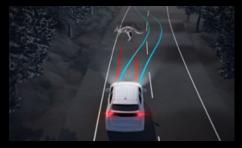
Anti-lock Braking System Mitsubishi's Anti-lock Braking System allows the driver to maintain steering control of the vehicle and manoeuvre around obstructions in heavy braking situations.
