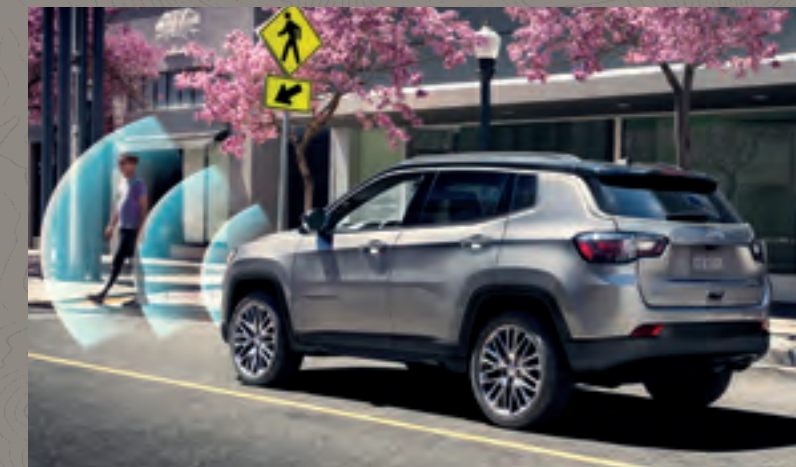
PEDESTRIAN / CYCLIST EMERGENCY BRAKING 15 Drivers are provided a warning and the vehicle automatically decelerates to help avoid an impending collision with a pedestrian or cyclist ahead. Standard.
