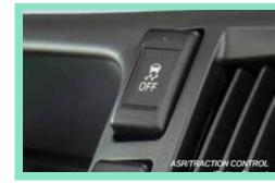
When the ESC system senses that the driver is at risk of losing control of the vehicle, it alerts the driver with an on-dash warning light, reduces engine output, and applies braking pressure as needed. ESC works in tandem with ASR, an advanced tractioncontrol system that provides tire grip when the truck is on loose, wet, or slippery surfaces.
