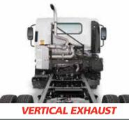
For custom body mounting and special equipment, exhaust is relocated from the frame rail to directly behind the cab. Available on N-Series Diesel Standard Cab only.
