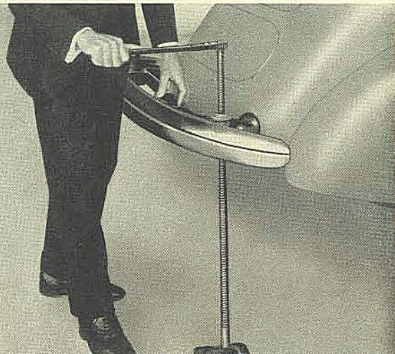
Easy Jacking System. —Chevrolet's new system of jacking takes all the fuss and bother out of raising the car. There's no necessity to stoop or bend — it is so simple that it can be operated by a child. This jack is designed to raise the car by means of the bumper bar supports at the front and rear of the car instead of difficult-to-get-at jack pads underneath the car. To jack up a wheel you simply hold the jack upright on the ground with the jacking bracket head (with its specially designed grip) under the bumper bar support nearest to the wheel — then, standing in an upright position, you merely operate the jack handle (which works on the ratchet principle) with an easy to and fro motion — a few turns and the car is raised, lifting the wheel free of the ground.
