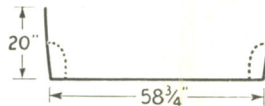
Chevrolet Open Utility —Max. width of body at floor line, 4 ft. 10 1/2 in.; taildoor opening, 3 ft. 11 1/2 in.; max. floor length, 7 ft.; height of sides (floor to top of sides), 1 ft. 8 in. Standard equipment includes a neat "snap on" waterproof cover for the load compartment when it is not in use.
