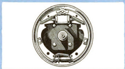
New Jumbo-Drum Brakes . . . As much as 25% less pedal pressure is required with these completely new brakes. Lining area is increased 15% in wider front brakes. Brake life is longer.
