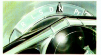
The pointer on the illuminated Hydra-Matic quadrant shows at a glance the driving range selected.
