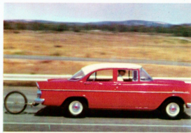
(1) The "8th wheel" measures Holden's outstanding petrol economy on the Proving Ground Speed Loop. (2) Carefully measured grades are used to test Holden's willing power and excellent top gear flexibility. (3) The mile of Proving Ground travel is estimated to equal four miles of ordinary owner operation.
