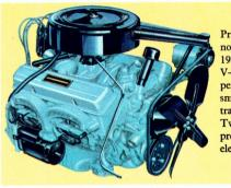
Proved, powerful and economical... the 283 cubic inch, 195-h.p. Chevrolet Turbo-Fire V-8 engine combines spirited performance with exceptional smoothness and quietness, plus traditional Chevrolet economy. Two-barrel carburettor, full-pressure lubrication and dry element air cleaner are standard.
