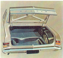
Big, new 26.4 cu. ft. boot has a lower loading height, deep floor well for bulky items. Wheel can be removed without disturbing luggage. Fuel tank now holds 11.5 gallons.
