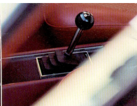
4 on the floor Gentlemen with the gift of the grab will specify an all-synchro 4-speed box with stick shift in a sporty console.
